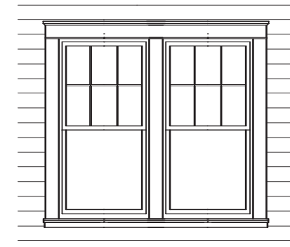
Mullion window has 5/8" trim (mullion) between frames. Double or triple mullion windows are acceptable.
